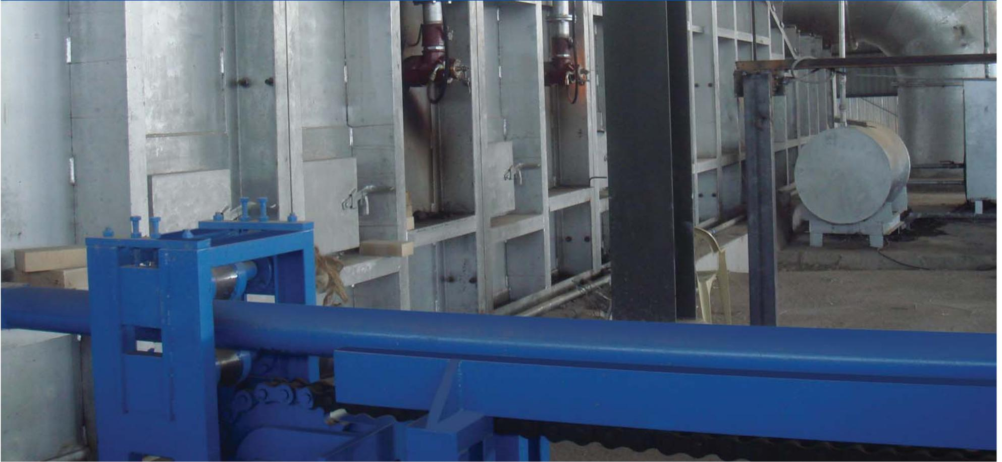
A 30 ton/hr capacity reheating furnace in our rolling mill tempers the internally produced billets and sends them to the flow for the production.
