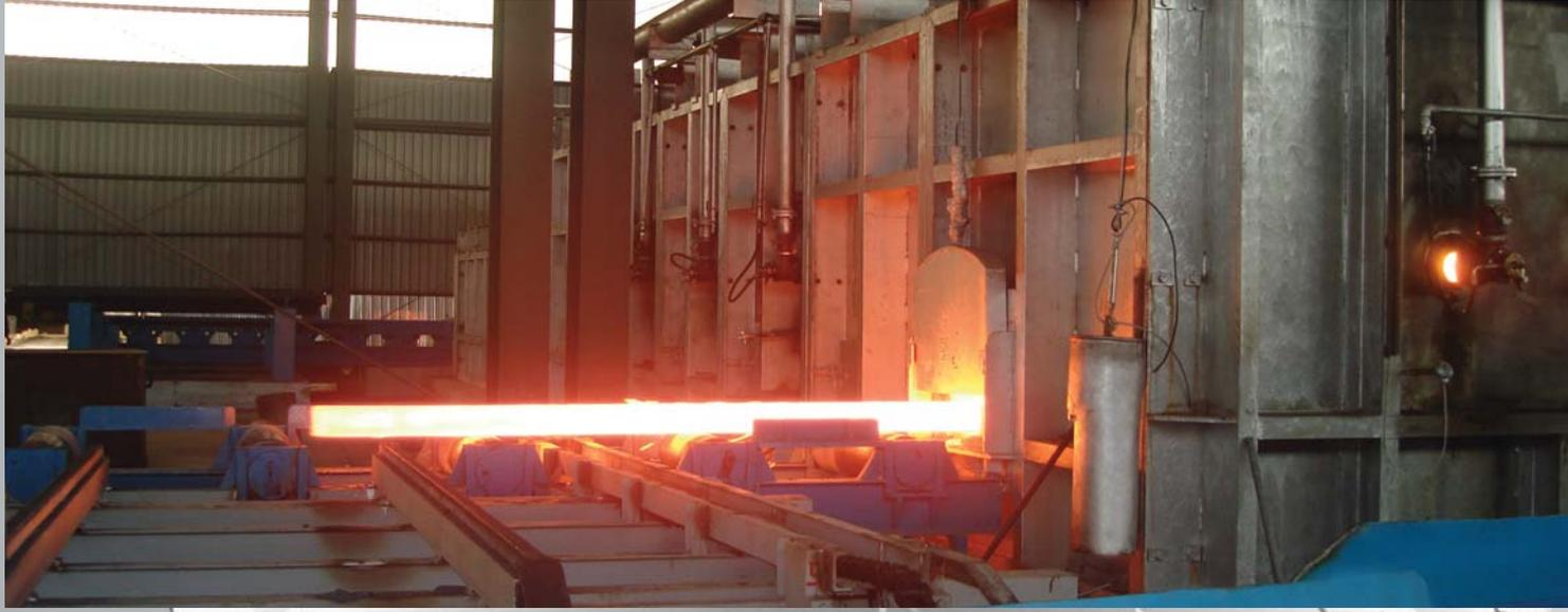
This unit consists of 3 group preparation benches, 42 meter long natural cooling grill, and a cold cutter with a capacity of 250 tons.
